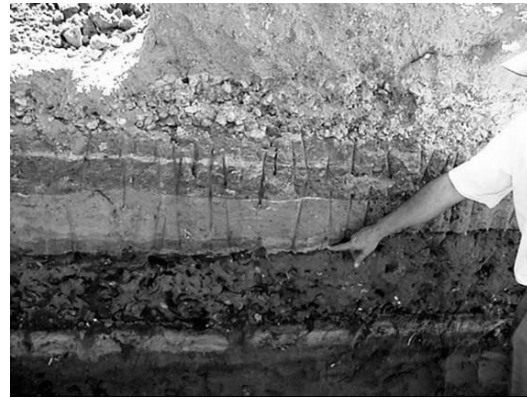
Figure 2. Prothrombolithic stratum located below the non-consolidated superficial beach stratum in the CICIMAR-IPN foundation site.
